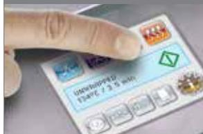
A large touch screen offers communication between the unit and the user, allowing for easy operation, and tutorial viewing.
