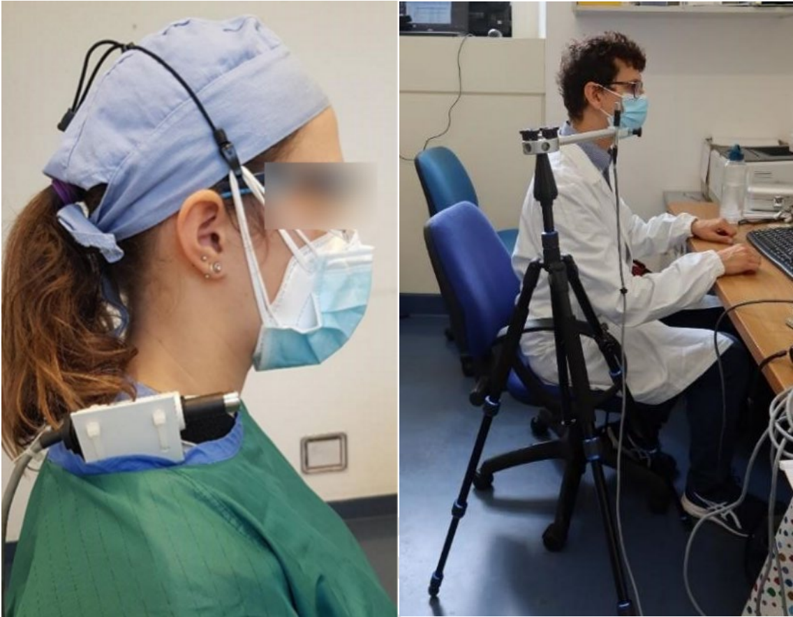
FIGURE 1: MICROPHONE PLACEMENT FOR DOSIMETRIC MEASUREMENTS
